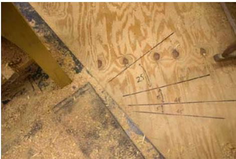
The handle of the tool can reference these lines to make sure the expected angle is being used.
