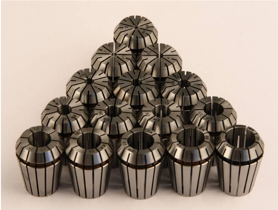
A set of ER25 metric collets (2mm to 16mm)
