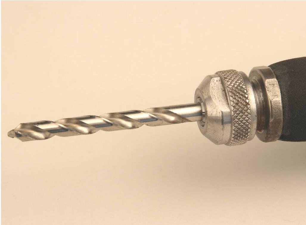
ER collets can be sourced to suit various round shaft tools
